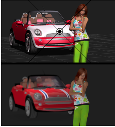
The Focus Distance control, with Alyson as the point of focus, and its render.
